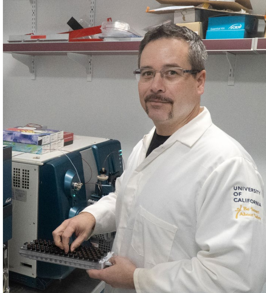
Faculty member Luke Wittenburg with the tandem mass spectrometer, which is used to measure drug concentrations in fluid and tissue samples for pharmacokinetic analysis. Photo: Mike Bannasch
